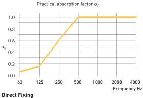
Thickness: 40 mm Absorption Class: A
